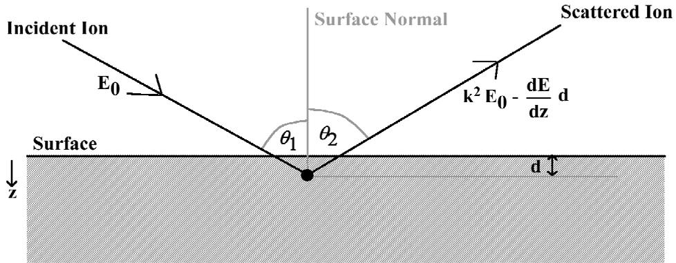
Figure 3.5: The energy loss due to inelastic scattering becomes greater the deeper the ion penetrates. An ion entering the crystal with energy  $E_0$  and being scattered at a depth  $d$  from the surface exits with energy given by Equation 3.9.
