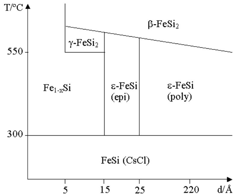
Figure 6.1: Bulk phase diagram for Fe silicide. After von Kanel et al. [15]. The FeSi system exhibits many phases in the bulk dependent on the precise Fe:Si composition and sample preparation.
