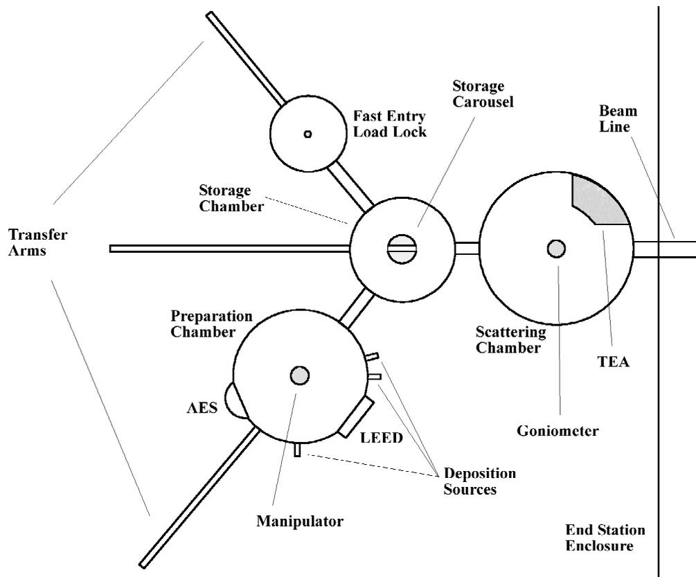
Figure 2.2: Schematic diagram of the Daresbury MEIS facility user end station. The ion beam enters at the main scattering chamber. Sample preparation is performed in a separate chamber and sample storage and fast entry is also available.
