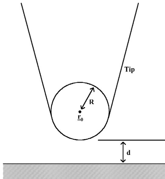
Figure 2.5: The model tip used in the calculations of Tersoff and Hamann [13, 14]. The tip is taken as a spherical potential well of radius  $R$ , centred at  $\mathbf{r}_0$  a distance  $d$  above the surface.
