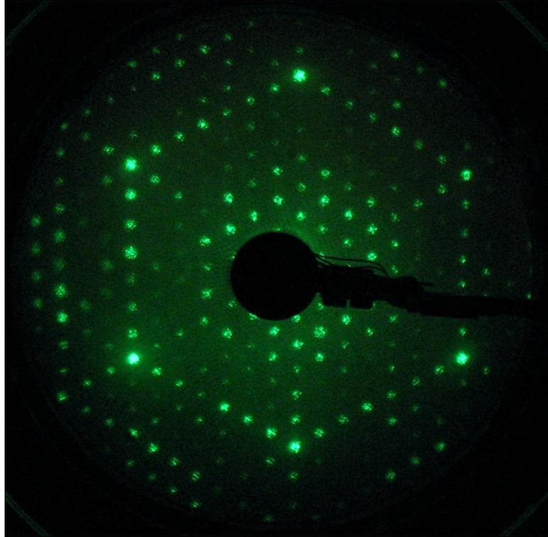
*Figure 2.12: An example LEED pattern [24], showing the diffraction pattern from the clean Si (111)  $7 \times 7$  surface with incident electron energy of 40 eV. Note that the periodicity of the surface is immediately apparent.*
