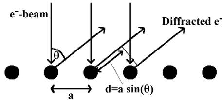
Figure 2.10: Simple diffraction in 1D. Constructive interference occurs when the Bragg condition is met, i.e. path difference  $d = n\lambda$ ,  $\lambda$  being the electron wavelength and  $n = \dots -2, -1, 0, 1, 2, 3, \dots$
