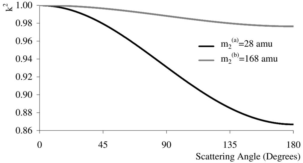
Figure 3.3: The kinematic factor  $k^2$  as a function of scattering angle for two target masses of 28 amu and 168 amu, calculated for the case of  $H^+$  ions.
