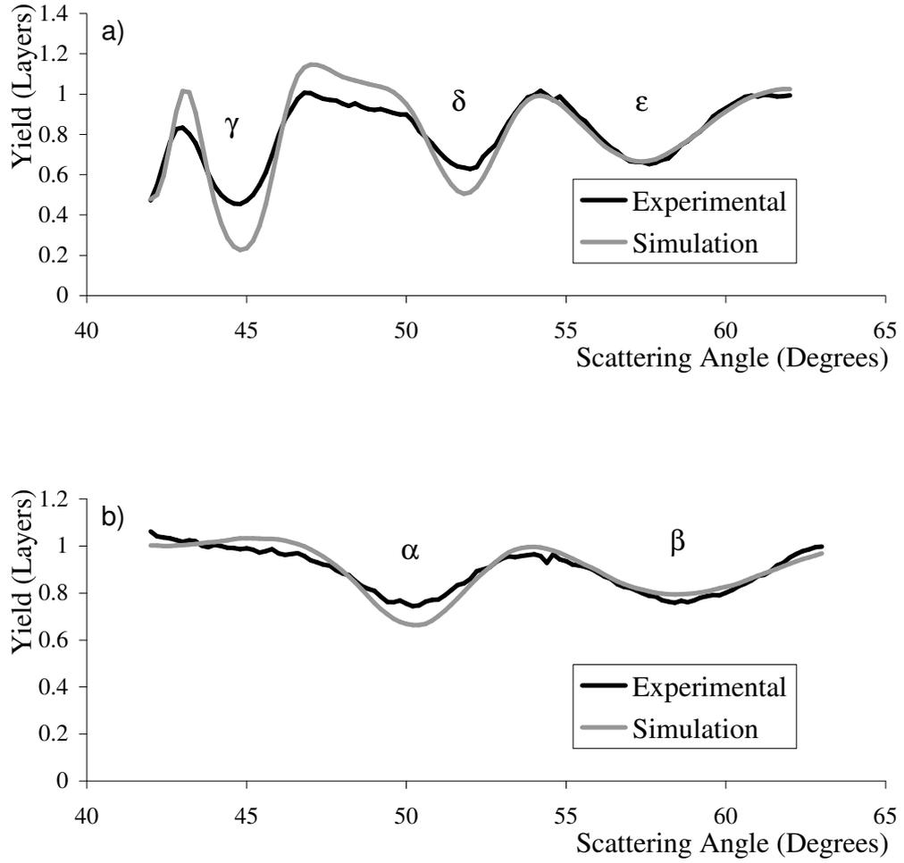
Figure 4.10: Comparison between experimental data and simulation for the “by eye” fit, corrected for Rutherford scattering cross-section. (a)  $[1\bar{1}00]/[1\bar{1}11]$  (b)  $[1\bar{1}\bar{1}]/[100]$ . The  $\sim 57^\circ$  ( $\epsilon$ ) dip position has been further improved.
