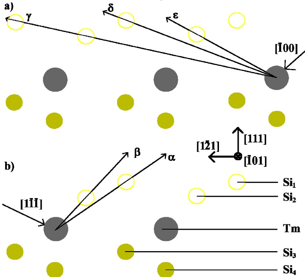
Figure 4.2: The origin of the blocking dips in the Tm signal in the two scattering geometries indicated. a)  $[\bar{1}00]/[\bar{1}11]$  b)  $[1\bar{1}\bar{1}]/[100]$ . The arrows indicate the origin of the blocking features labelled in Figure 4.5. Refer to Figure 4.1 for further details of the structure (note that in this figure only those atoms within the scattering plane are shown). Notice that  $\epsilon$  depends only on  $Si_2$ .
