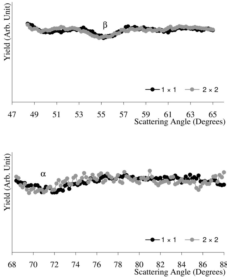
Figure 6.4: Comparison of scattering curves from the  $1 \times 1$  and  $2 \times 2$  phases.  $[\bar{1}00]/[\bar{1}11]$  geometry. The scattering curves from the two phases are extremely similar, indicating that their structures are very alike. See also Figure 6.5 and Figure 6.6.
