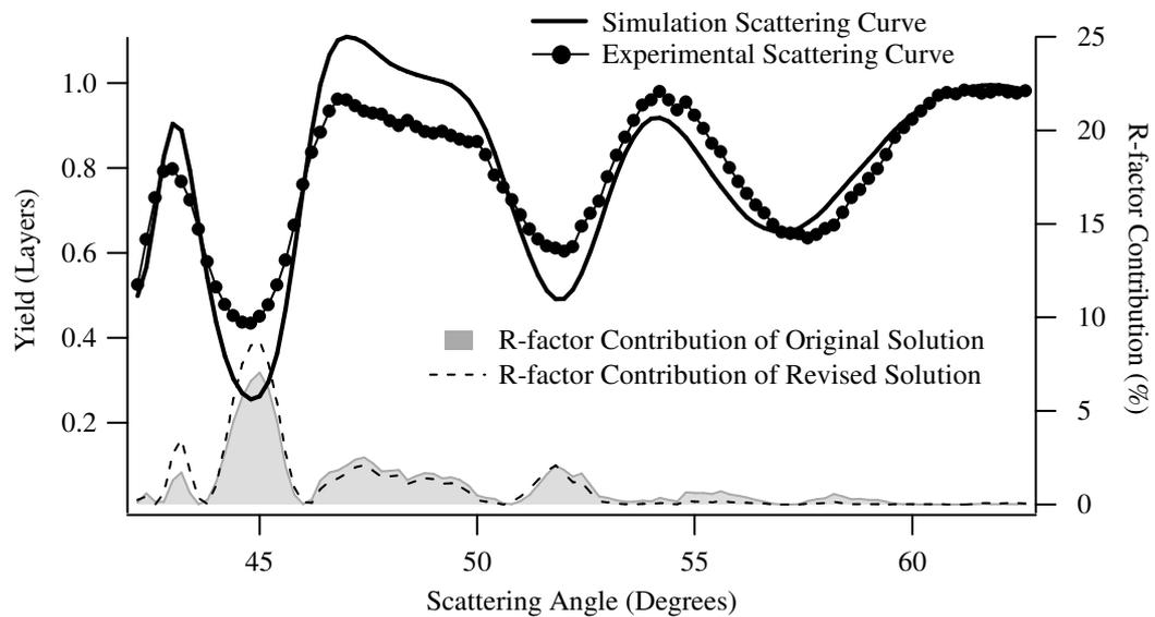
Figure 5.5: Contribution of each point to the total R-factor when the Rutherford scattering cross section is not taken into account. This eliminates the added weight given to lower angles due to the additional number of counts. The depth of the lowest angle dip is still the most important factor.
