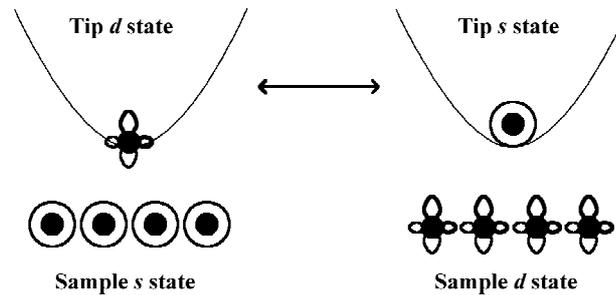
Figure 2.6: Qualitative description of the reciprocity principle. Probing surface  $s$  states with a tip  $d$  state is equivalent to probing  $d$  states with a tip  $s$  state.
