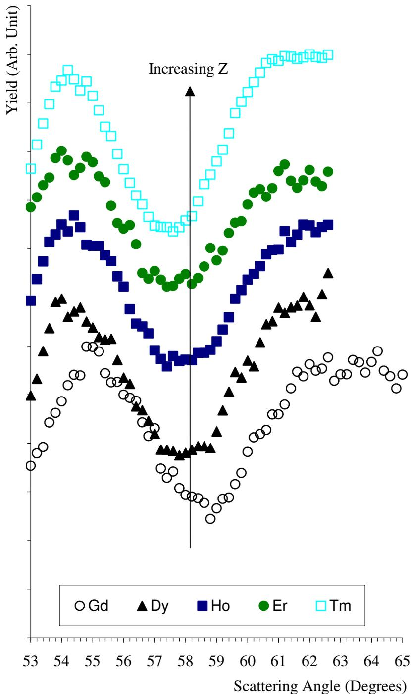
Figure 5.2: Comparison of experimental MEIS scattering curves for 2D rare earth silicides. This feature is due to the blocking of scattered ions by the  $\text{Si}_2$  atoms and directly reflects the  $\text{Si}_2$ -RE bond length (the blocking dip labelled  $\epsilon$  in the previous Chapter). Curves have been scaled to an arbitrary yield and then offset for clarity.
