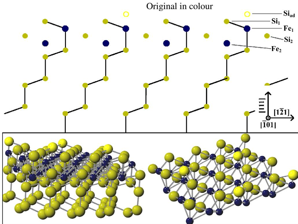
Figure 6.7: The proposed structural model for the initial Fe silicide growth. Side view showing the scattering plane. Note that the  $2 \times 2$  phase is shown; the  $1 \times 1$  phase is proposed to be identical but without the ordered Si overlayer,  $\text{Si}_{ad}$ . Inset: Ball and stick model of the surface—the model on the right has the bulk Si removed for clarity.
