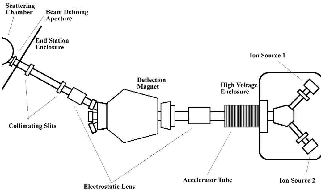
*Figure 2.1: Schematic diagram of the Daresbury MEIS facility beam line. Ions are produced by a duoplasmatron source and accelerated to around 100 keV. The ion beam is then focused and collimated before entering the scattering chamber.*
