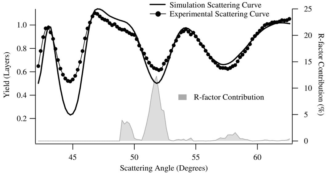
Figure 5.6: Contributions to the  $R$ -factor when discounting the lowest angle dip from the calculation of the  $R$ -factor. This produces a much better fit to the higher angle dips than that shown in Figure 5.4 and Figure 5.5.
