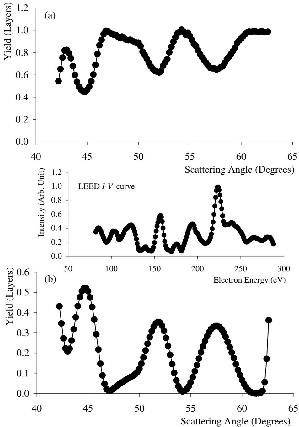
Figure 5.7: Comparison of (a) the original Tm silicide MEIS scattering curve and (b) the “flipped” version. The inset shows a typical LEED I–V curve [10]. The Pendry R-factor was originally designed to deal with peaks rather than dips. The flipped data may be considered qualitatively more like the LEED data for which the Pendry R-factor is standard.
