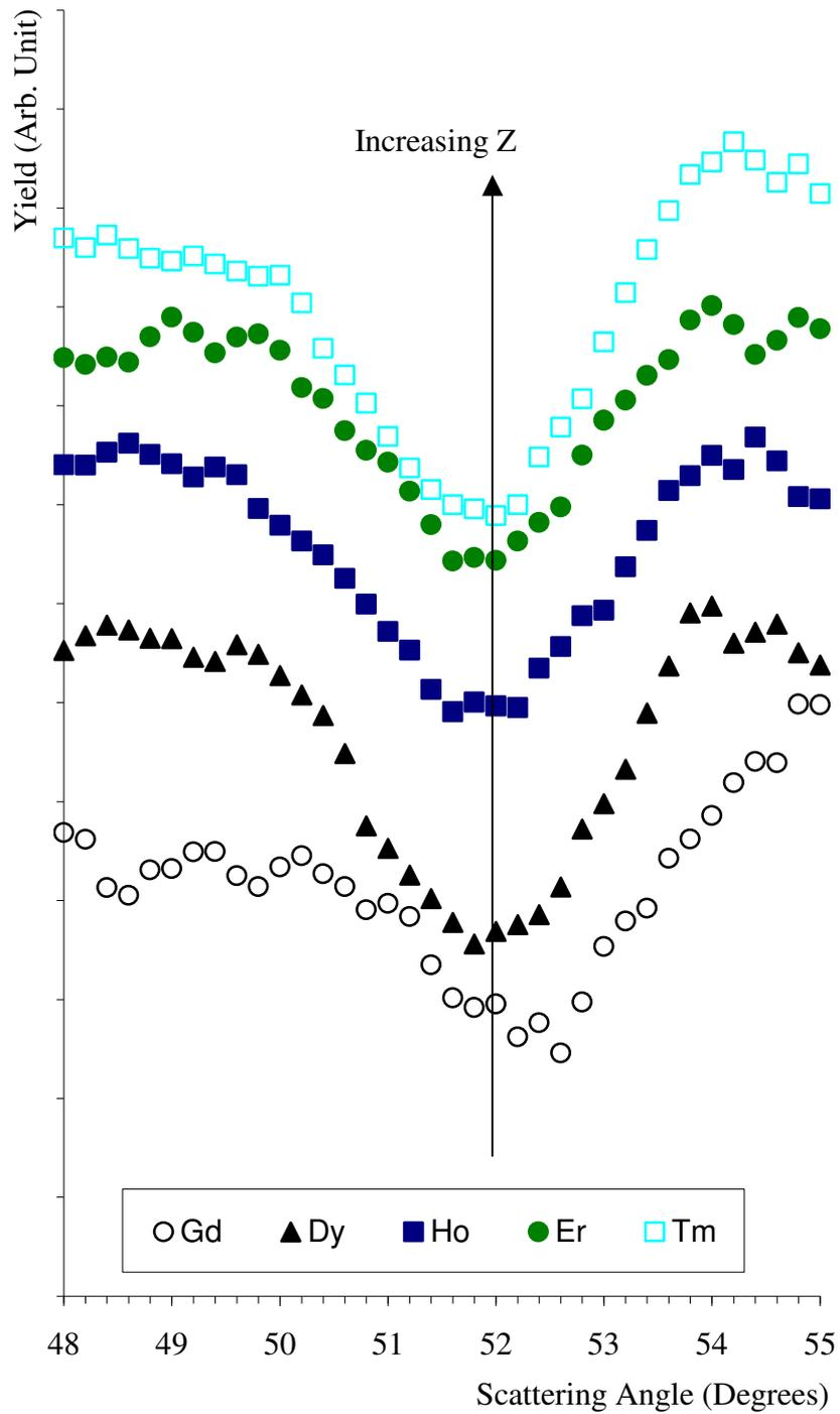
Figure 5.3: Comparison of experimental MEIS data for 2D rare earth silicides. The blocking dip shown is due to blocking of scattered ions by the  $Si_1$  atoms (the blocking dip labelled  $\delta$  in the previous Chapter). Curves have been scaled to a common arbitrary yield and then offset for clarity.
