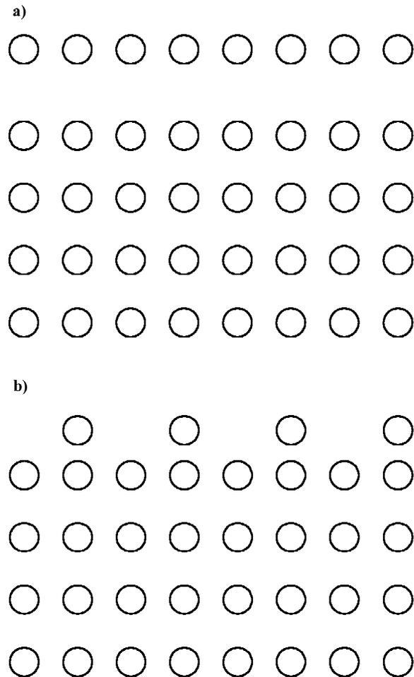
*Figure 1.1: Simplified side view of a) a surface relaxation in which the atomic spacing changes near to the surface; b) a surface reconstruction, in which the atomic arrangement reconfigures to produce a new two-dimensional unit cell.*
