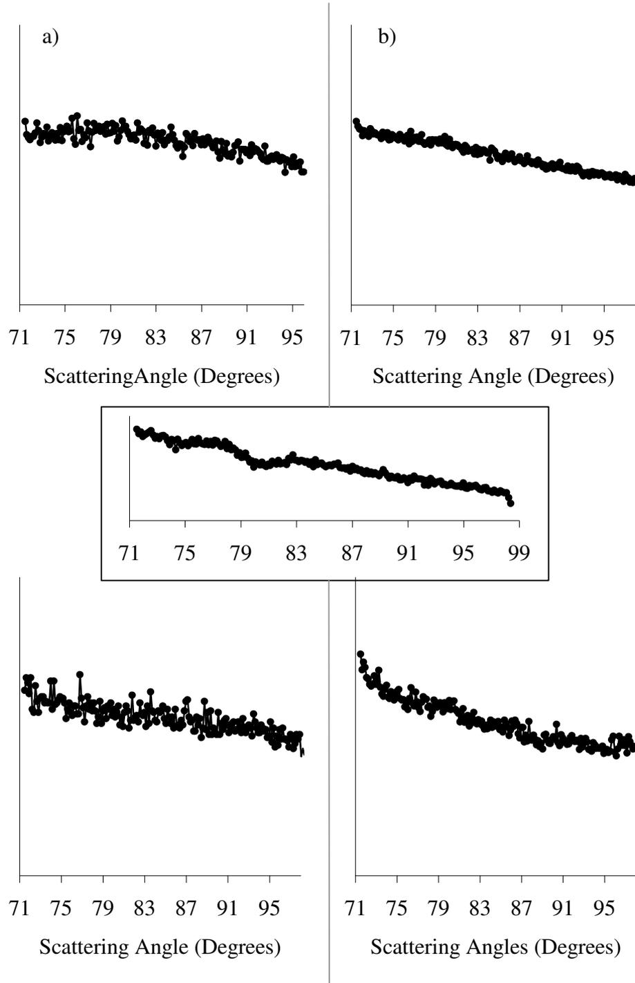
Figure 7.9: Scattering cross section through the Ho (top) and Fe (bottom) signals of spectra shown in Figure 7.8. a) As deposited b) After anneal to  $\sim 550$  °C. Inset: The scattering curve through the Ho signal before Fe deposition. The lack of blocking features in the Ho and Fe signals indicate a lack of order at the surface.
