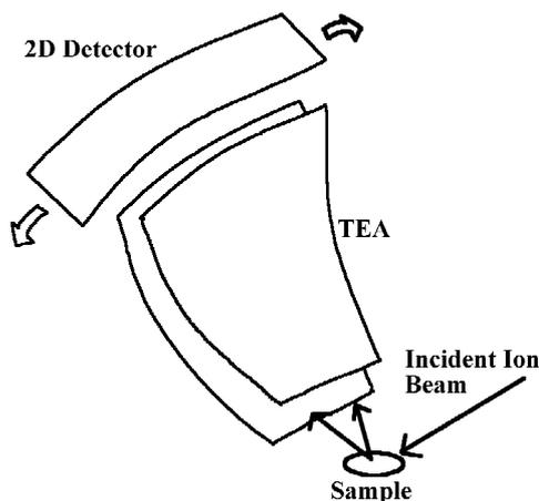
*Figure 2.3: The toroidal electrostatic analyser and 2D detector produce the 2D data sets in MEIS experiments. Ions entering the detector are bent through  $90^\circ$  before hitting a set of channel plates which amplify the charge so it may be detected by the 2D detector plate.*
