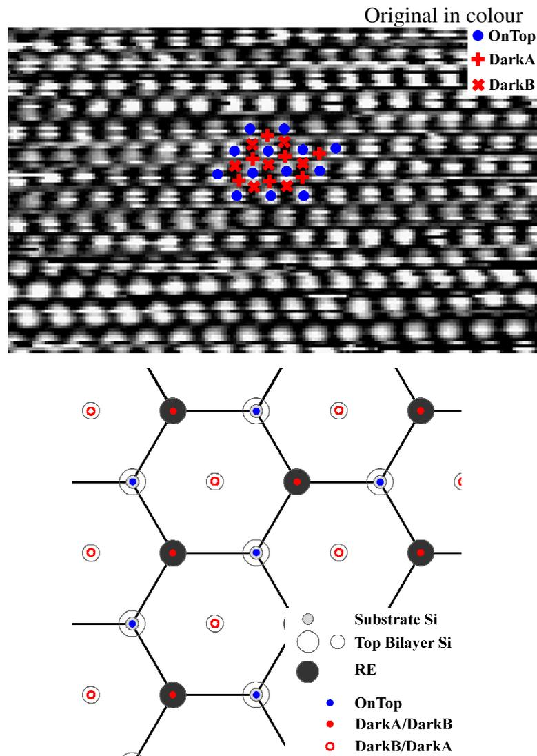
*Figure 7.3: Inequivalent sites on the 2D silicide surface. Top: atomically resolved STM image, bias voltage 2 V, tunnelling current 2 nA.  $\sim 5.0$  nm  $\times$   $\sim 3.6$  nm. Bottom: Schematic top view of the surface.*
