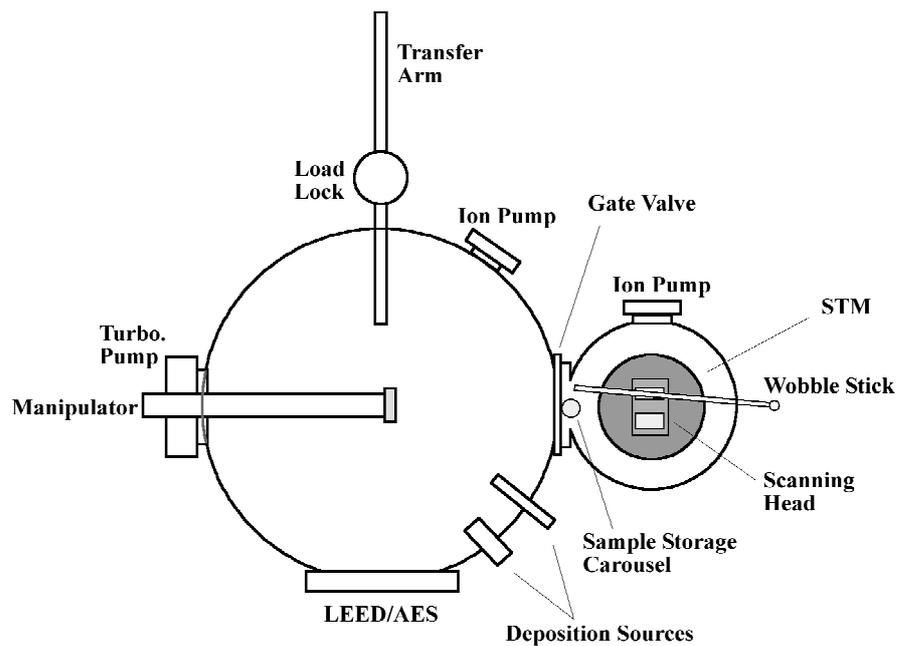
Figure 2.9: Schematic diagram of AFM/STM systems used. The UHV STM side chamber may be isolated from the main UHV sample preparation chamber. Samples may be quickly exchanged in and out of the system using a load lock
