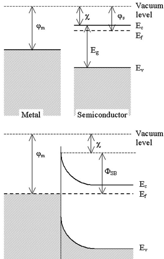
Figure 1.3: Formation of a Schottky barrier,  $\Phi_{SB}$ , for an n-type semiconductor in contact with a metal. The Schottky barrier forms, and the junction is rectifying, if the metal work function,  $\phi_m$ , is greater than the semiconductor workfunction,  $\phi_s$ .  $E_v$  is the top of the valence band,  $E_c$  the bottom of the conduction band and  $E_f$  the Fermi level. The band gap of the semiconductor,  $E_g$  is also indicated.
