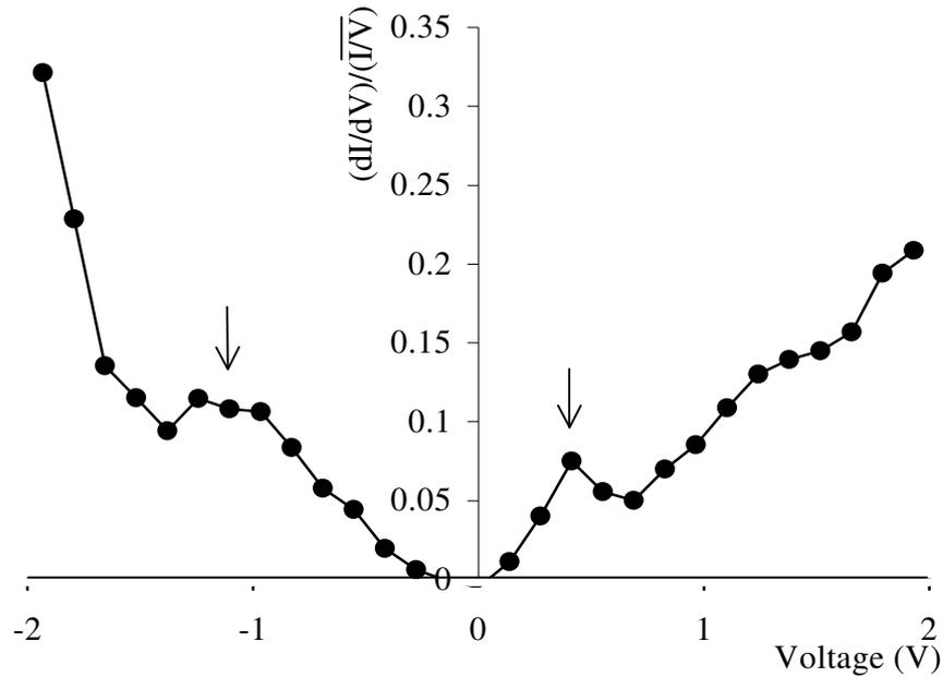
Figure 7.5: The LDOS is better represented by a plot of  $(dI/dV)/(I/V)$  versus bias voltage. Arrowed are features corresponding to bands in the 2D silicide band structure
