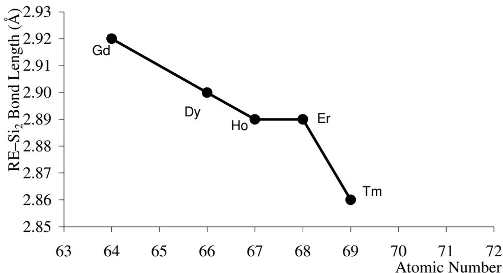
*Figure 5.8: The structural trend in the Si<sub>2</sub>–RE bond length across the rare earth series. This plot is derived from the structural model determined using  $R_{Pflip}$ . Other methods of determining the best fit model show a similar trend.*
