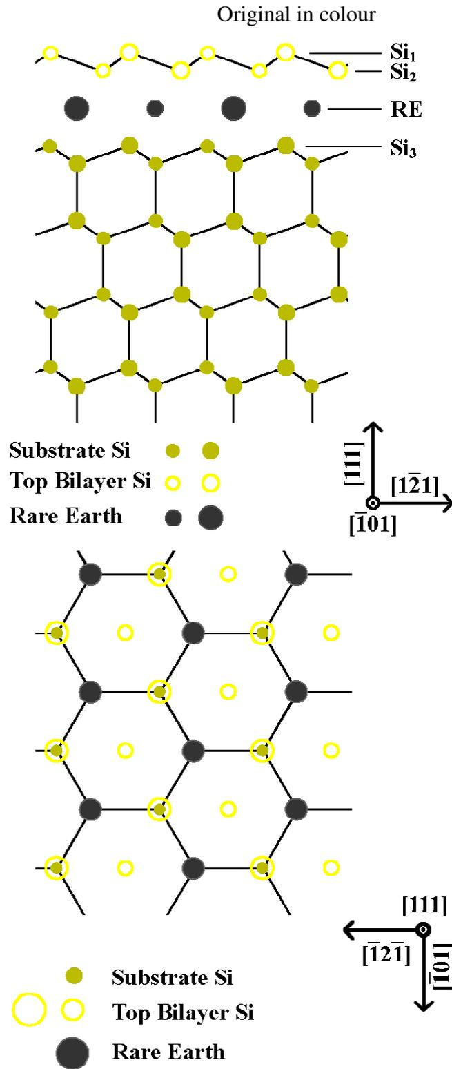
Figure 4.1: Structure of 2D rare earth silicides. The RE forms a single atomic layer located in T4 sites above the bulk Si. The silicide is terminated by a bulk-like Si bilayer ( $\text{Si}_1$  and  $\text{Si}_2$ ) which is rotated by  $180^\circ$  with respect to the bulk. a) side view, b) the view along the surface normal (i.e. top view).
