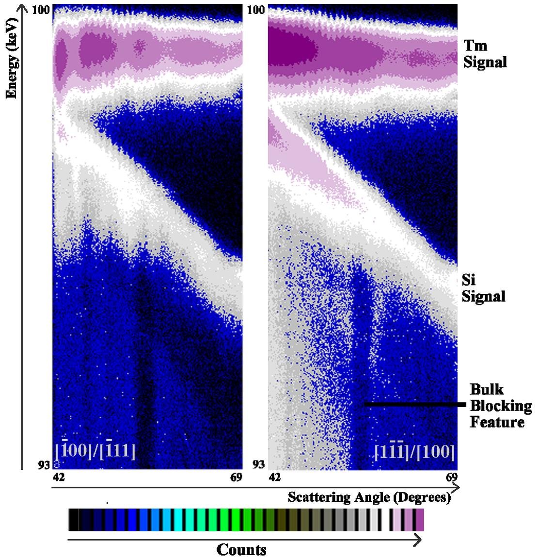
Figure 4.3: Typical MEIS spectra from the Tm silicide for the two experimental geometries employed (left  $[\bar{1}00]/[\bar{1}11]$ ; right  $[1\bar{1}\bar{1}]/[100]$ ). The separation of the Tm and Si signals, and the bulk blocking features are all clearly visible. The Tm signal shows decreased intensity at scattering angles at which blocking has occurred.
