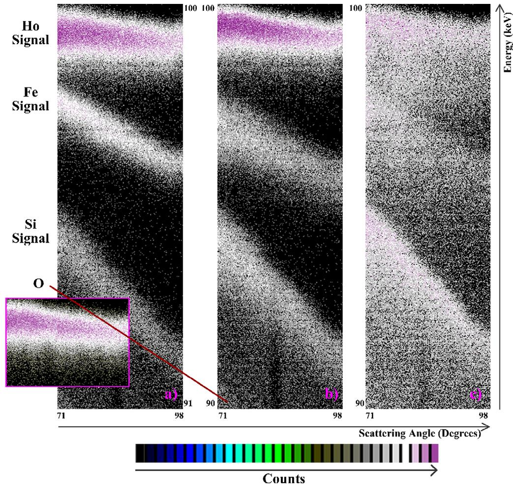
Figure 7.8: The sequence of MEIS spectra from Fe deposition on Ho 2D silicide.  $[1\bar{1}0]$  incident direction with detection around  $[100]$ . a) As deposited b) After anneal to  $\sim 550$  °C c) After anneal to  $\sim 700$  °C. The inset shows the Ho scattering signal from the 2D silicide before Fe deposition. The surface is initially disrupted and increasing annealing simply causes diffusion of the Fe and Ho into the bulk substrate.
