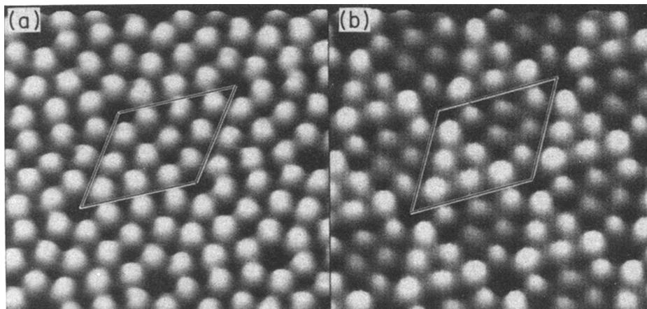
*Figure 2.7: Bias condition dependence of STM imaging, in the case of the Si(111)  $7 \times 7$  surface. (a) Unoccupied states with the sample biased at +1.5 V. (b) Occupied states with the sample biased at -1.5 V. The unit cell is marked in each case. Note that in the case of (b) a difference is clear between the faulted and unfaulted half of the unit cell, whilst in (a) the two halves appear the same. From Avouris & Wolkow [16].*
