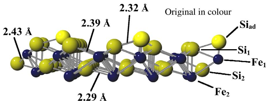
*Figure 8.2: Side view of the Fe silicide, showing the  $2 \times 2$  Si adatom layer and indicating bond lengths. Bulk Si has been omitted for clarity. The silicide is a CsCl-type structure with, in the case of the  $2 \times 2$  phase, an additional layer of Si adatoms in a  $2 \times 2$  arrangement.*
