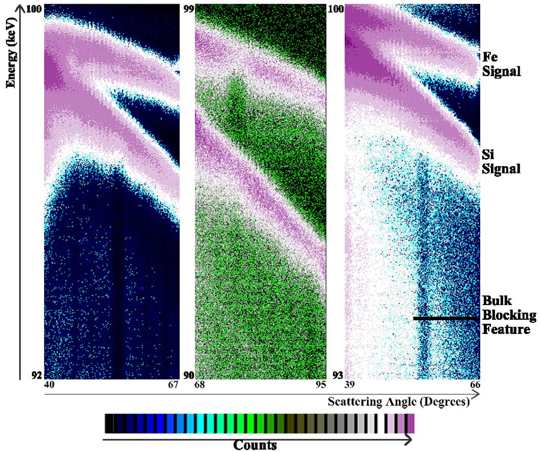
Figure 6.3: Typical MEIS spectra from the FeSi  $2 \times 2$  phase. Left to right:  $[\bar{1}00]/[\bar{1}11]$ ;  $[1\bar{1}0]/[100]$ ;  $[1\bar{1}\bar{1}]/[100]$ . The spectra are very similar to those observed for the  $1 \times 1$  phase (Figure 6.2).
