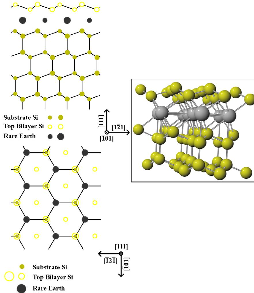
*Figure 1.4: Structure of the 2D RE silicides. The RE forms a single atomic layer situated in T4 sites above the bulk Si. The silicide is terminated by a bulk-like Si bilayer, rotated by 180° with respect to the bulk. Top: Side view. Bottom: Top view (i.e. along the surface normal). Inset: Ball and stick model of the surface.*
